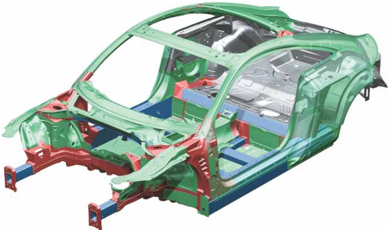
Sill section Audi TT Four-chamber extruded section
